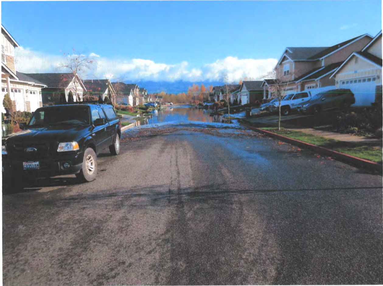
Photo 6. November 16,2021. Kent Turner. Looking east down Autumn Way. Note flooding in road and on sidewalks at low point in road in vicinity of two storm drains. This flooding was not contiguous with the adjacent flooded areas.
