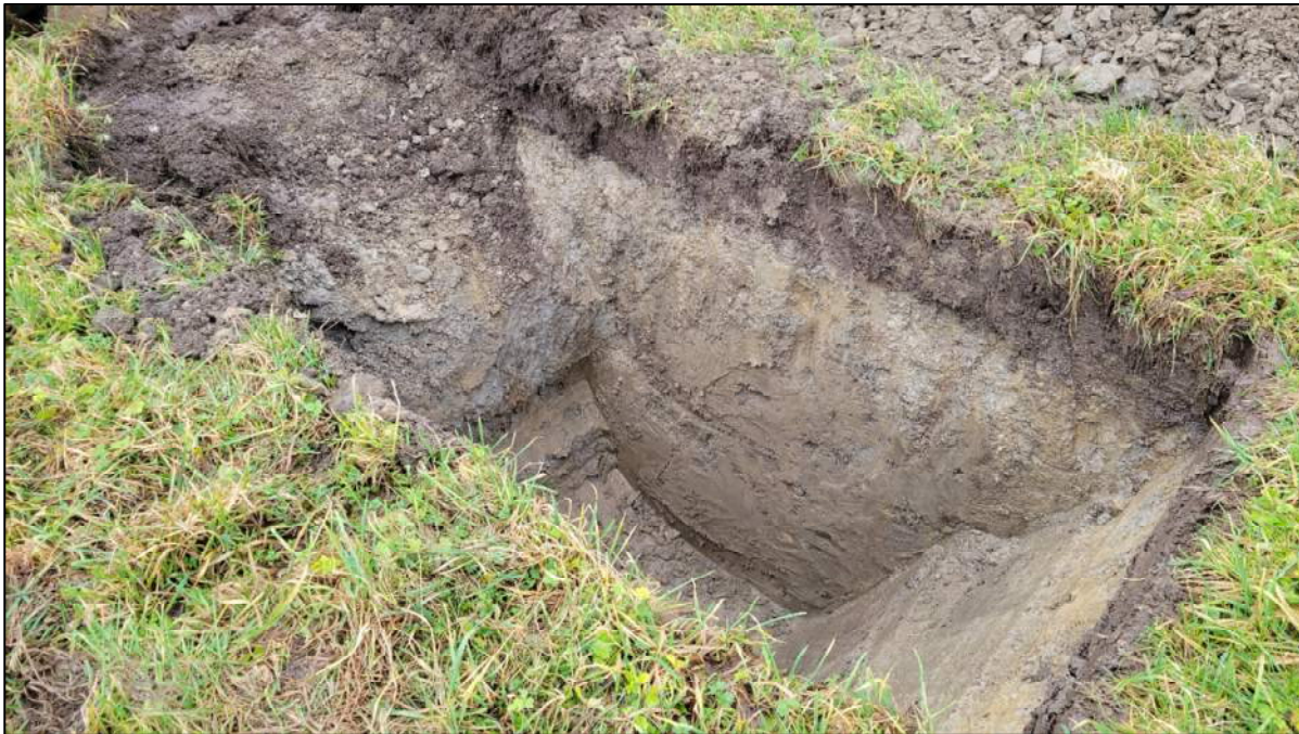
Image 2 – Typical subsurface soil profile showing 1-foot of topsoil overlying native soils. TP-2 shown in photo.
